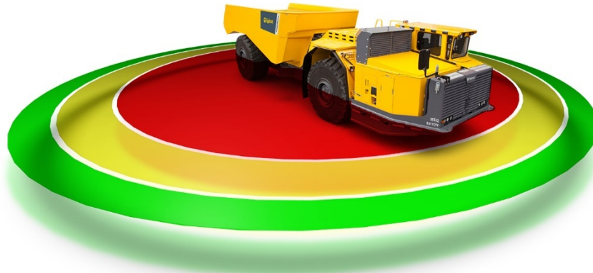
Figure 13 Epiroc MT42 with example visualization of near vehicle safe zones, with a green zone considered safe, a yellow zone of medium risk, and a high-risk red zone.
