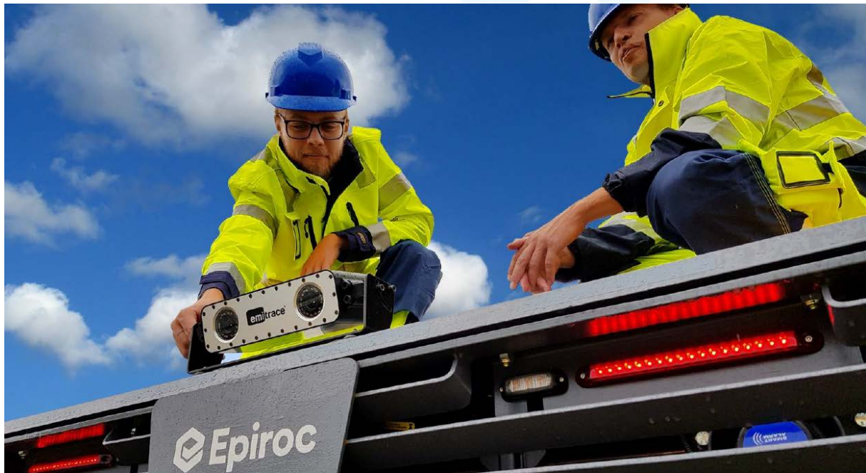
Figure 10 Emitrace® sensor system mounted on an Epiroc mine truck.
