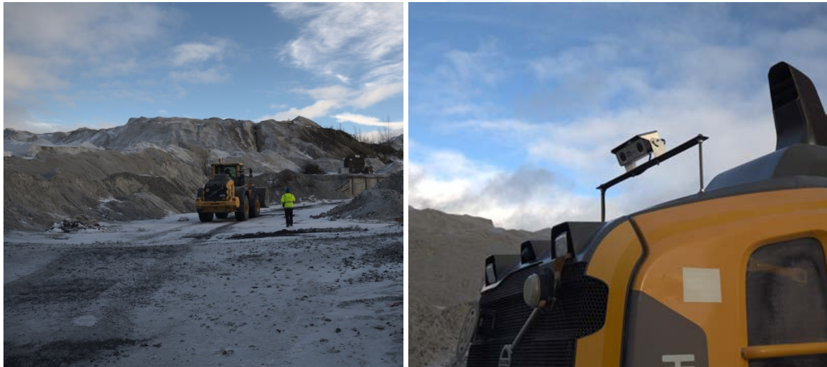
Figure 14 Evaluation of the emitrace® vision system on a wheel loader operating in an open-pit limestone quarry.
