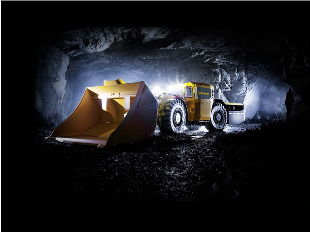
Figure 6: The Scooptram ST14 loader equipped with a streaming data unit. The unit will be utilised for collecting data in the illuMINEation project.
