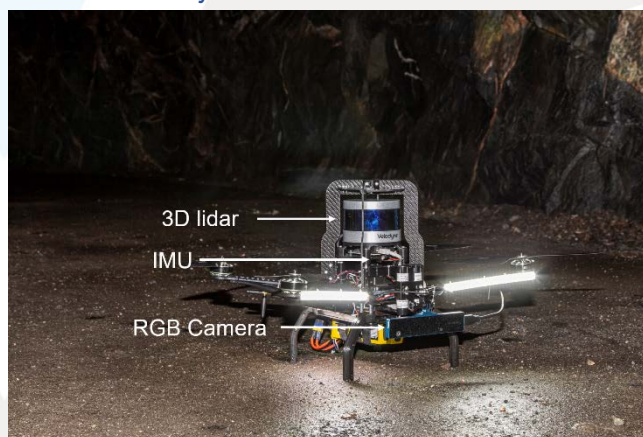
Figure 18 The drone equipped with IMU, RGB camera, and 3D lidar.
