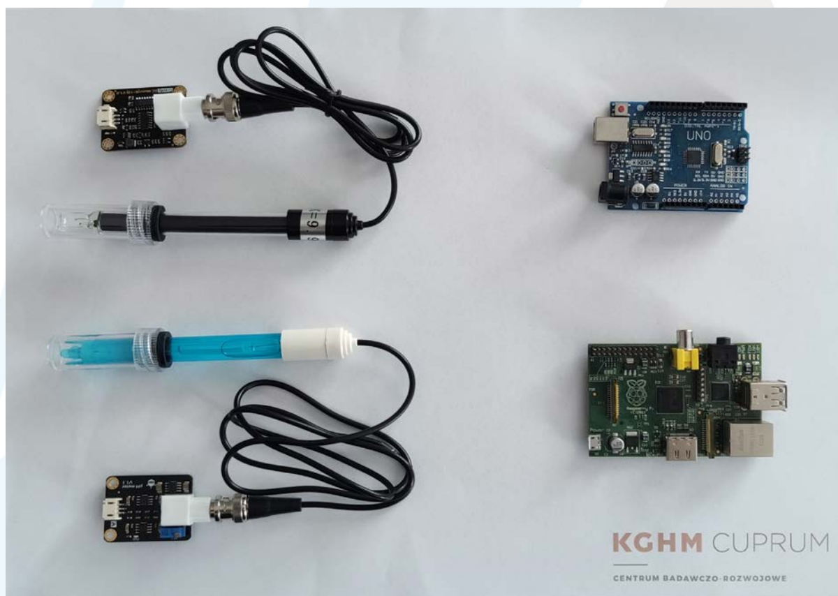
Figure 14 Sensors and microcontrollers. Upper left – electrical conductivity sensor, lower left – pH sensor, upper right – Arduino Uno, lower right – RaspberryPi
