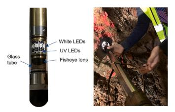
**Fig. 3.** Bottom part of the logging tool (left) and final stages of borehole surveying with the forward centralizer and the glass tube inside the hole (right).
