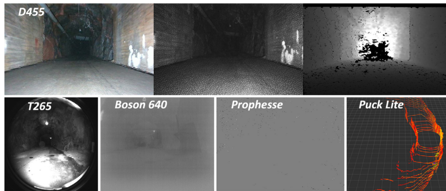
Fig. 1. Sample data output from the Luleå underground tunnel, collected with the Intel RealSense D455 camera — first row. In the second row are shown data outputs from an Intel RealSense T265, a thermal camera FLIR Boson 640, a Prophesse event camera and a 3D lidar Velodyne Puck Lite.
