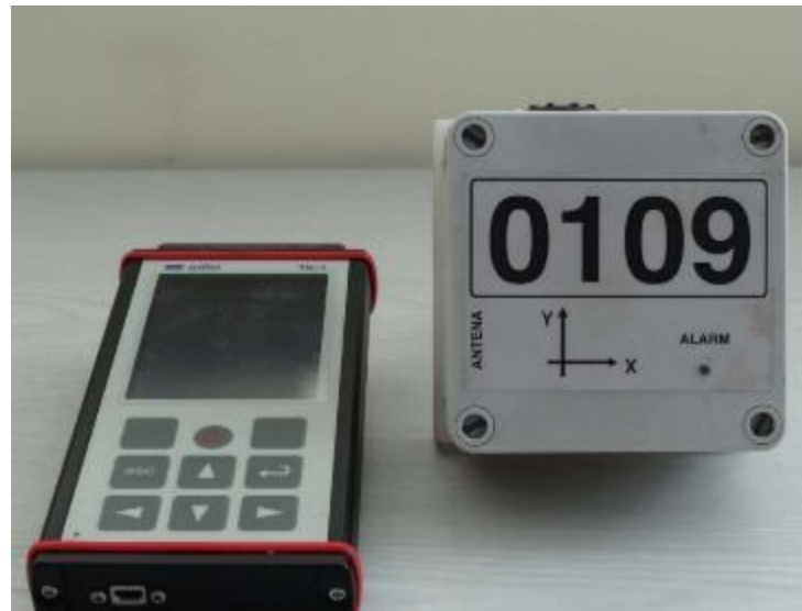
Figure 10. Inclinometric sensor with a wireless data transmitter.
