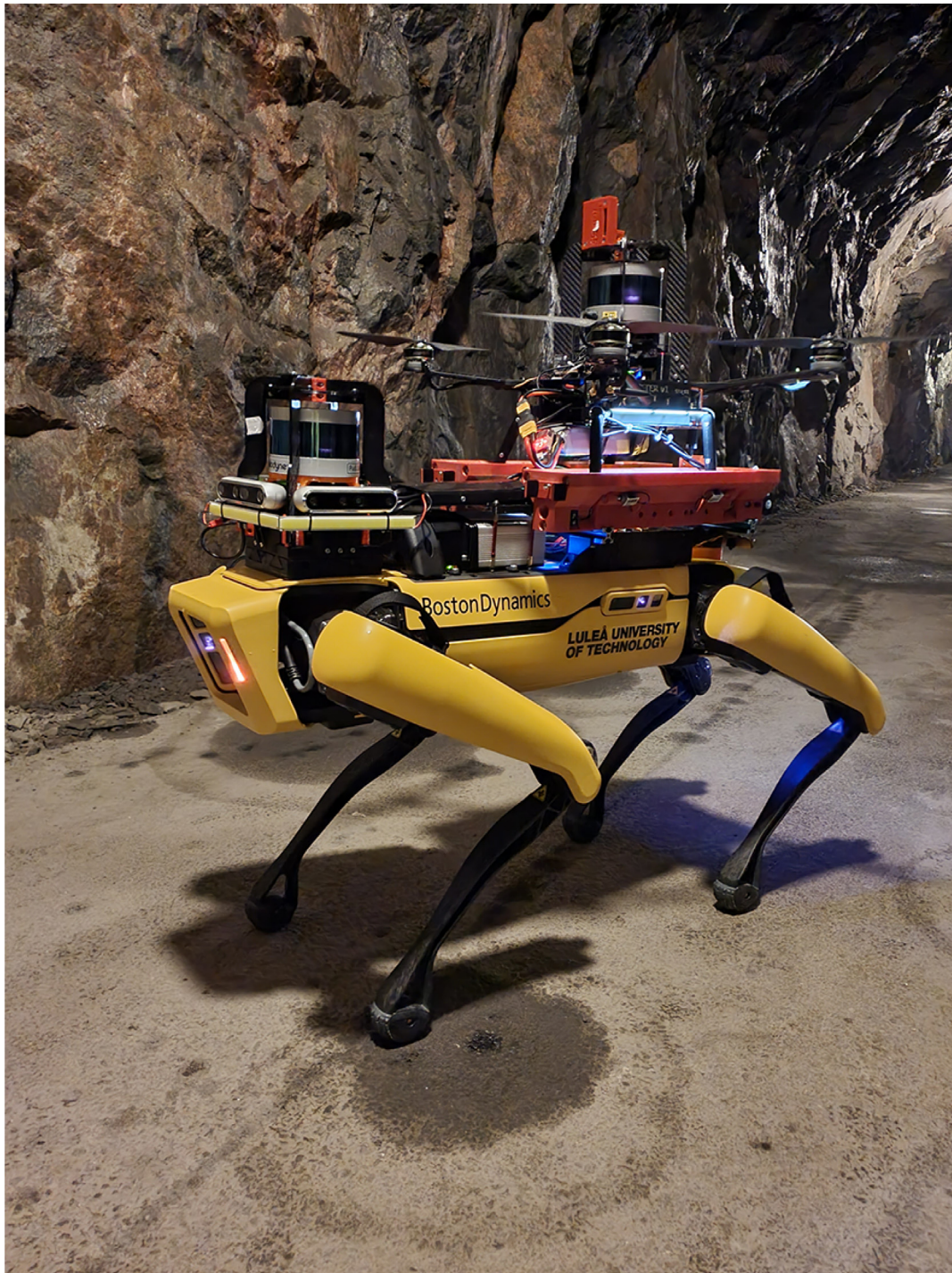
Fig. 2. The legged-aerial explorer with its full sensor suite and the UAV carrier platform.
