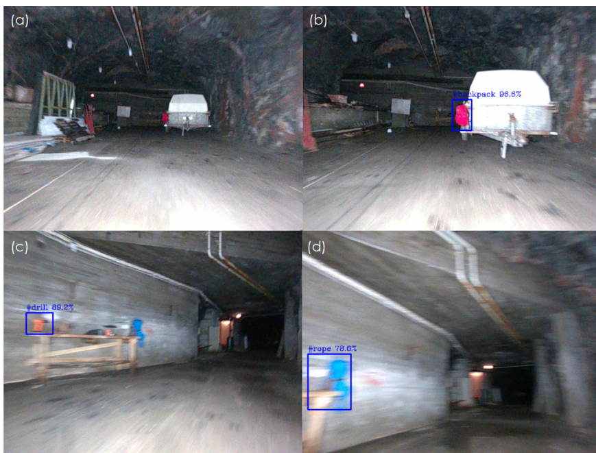
Fig. 15. Snap shot of the forward direction mission. (a) Static obstacles along the course, (b) backpack artifact detection, (c) drill artifact detection, (d) rope artifact detection.
