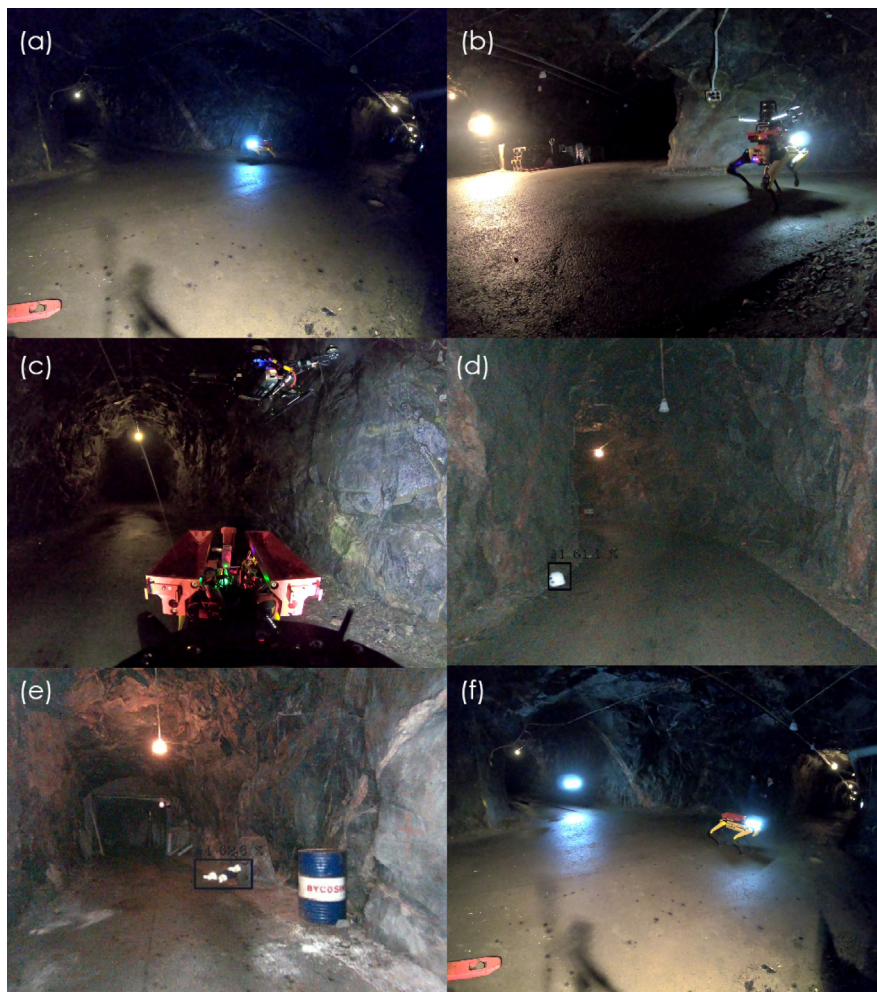
Fig. 12. Snap shots from the full mission. (a) Multimodality system approaching deployment point, (b) deployment point reached, (c) aerial agent take-off, (d) hard hat detection from onboard camera during COMPRA mission, (e) survivor detection, (f) aerial agent return to deployment point.
