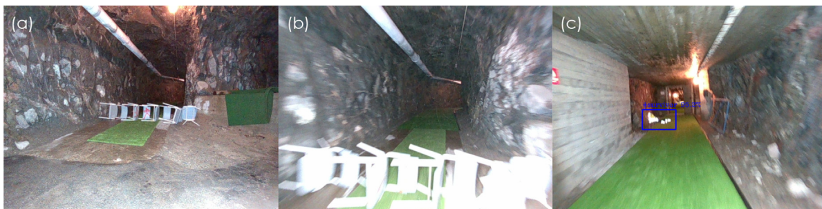
Fig. 17. Snap shot of the left direction mission. (a) Blocked passage for the legged robot, (b) UAV navigating above the blocked passage, (c) survivor artifact detection.
