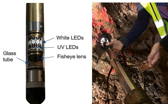
Fig. 3. Bottom part of the logging tool (left) and final stages of borehole surveying with the forward centralizer and the glass tube inside the hole (right).
