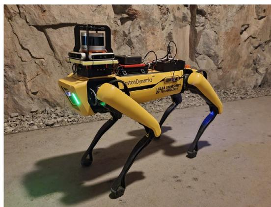
Fig. 2. The quadruped robot, Boston Dynamics Spot, that was used in experiments.
