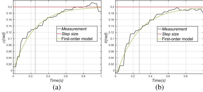
Fig. 11. System identification for the first-order time constants of LTU-Pixy. (a)  $\phi$  step response. (b)  $\theta$  step.
