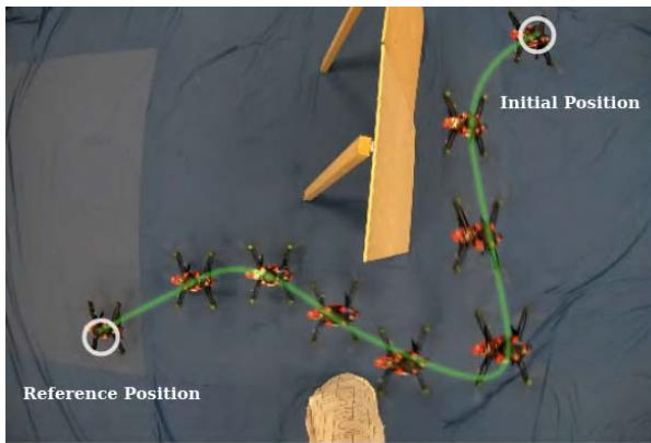
Fig. 14. Obstacle avoidance through a small opening.
