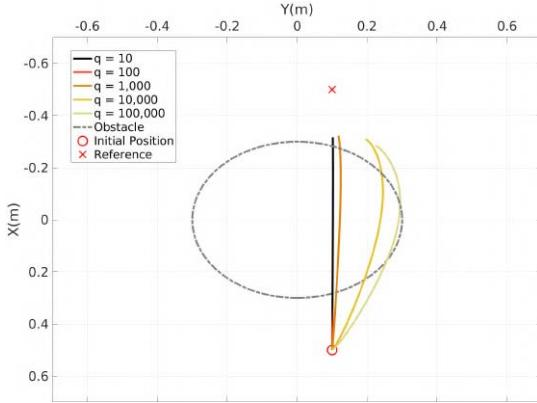
Fig. 5. NMPC optimized trajectories using one to five penalty method iterations for a circular obstacle with radius  $r = 0.3$  m. The cost minima are gradually pushed out as the cost associated with violating the constraint is increased.
