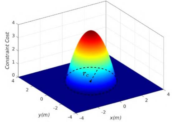
Fig. 2. Cost map of cylinder with radius 2 m.
