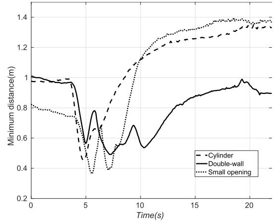
Fig. 21. Minimum distance from any obstacle by the closest LiDAR range measurement during the three experiment scenarios for the NMPC-based approach.
