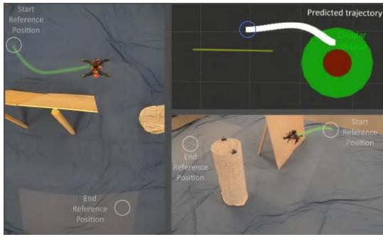
Fig. 28. Image from the third experiment, showing the nonconverged solution produced at 5.2 s into the small-opening experiment in Fig. 17.
