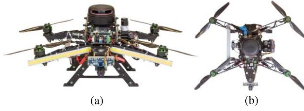
Fig. 7. UAV utilized for laboratory experiments. The subterranean scout, named the Pixy. (a) Front view. (b) Top view.
