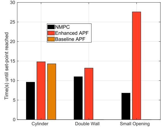
Fig. 15. Time duration from initiated movement until reaching the reference for NMPC and APF comparison.
