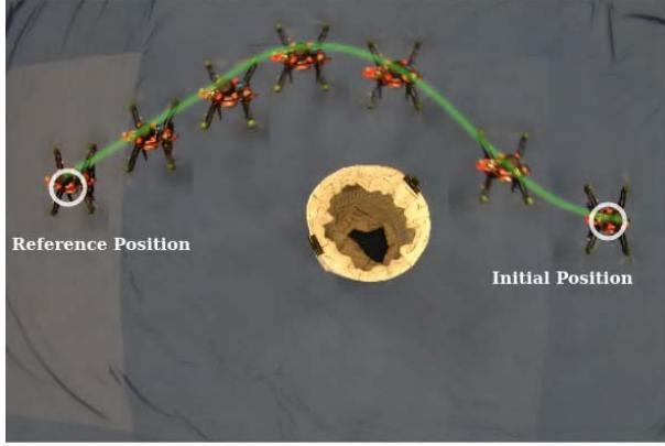
Fig. 12. Avoidance of a circular obstacle.
