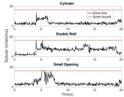
Fig. 16. NMPC-module solver time for the three experiments.
