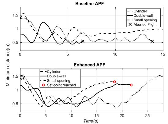
Fig. 22. Minimum distance from any obstacle by the closest LiDAR range measurement during the three experiment scenarios for the two APF approaches.
