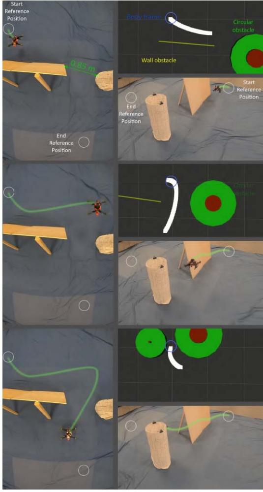
Fig. 25. Snapshot images from the third experiment. The UAV is tasked to move to the set-point reference, where the free path is a small constrained opening of 0.85 m between two obstacles. Using a safety radius of 0.4 m, the UAV can precisely pass through with an aggressive turn (within the dynamic constraints).
