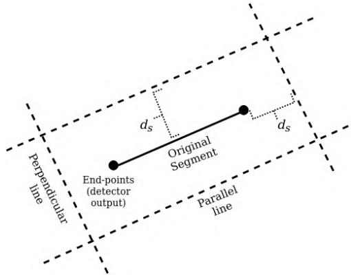
Fig. 3. Four lines envelop a line segment, with safety distance  $d_s$ .
