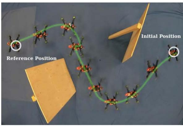
Fig. 13. Avoidance of two wall-like obstacles.
