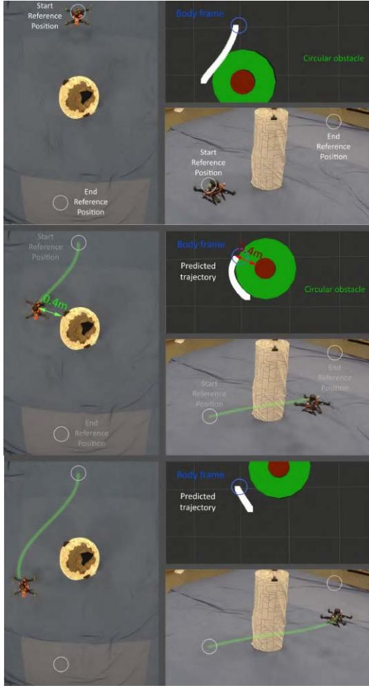
Fig. 23. Snapshot images of the first experiment. The UAV is tasked to avoid a cylindrical obstacle while performing set-point tracking. The maximum size radius of the UAV is 0.3 m; as such, we set the safety distance to 0.4 m.
