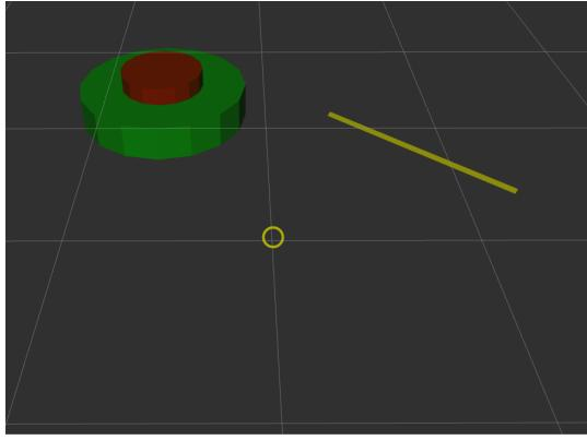
Fig. 9. Output from the obstacle detector in rviz from the scenario shown in Fig. 8, showing the radius and safety radius of the circular obstacle and the line segment from the wall-type obstacle.
