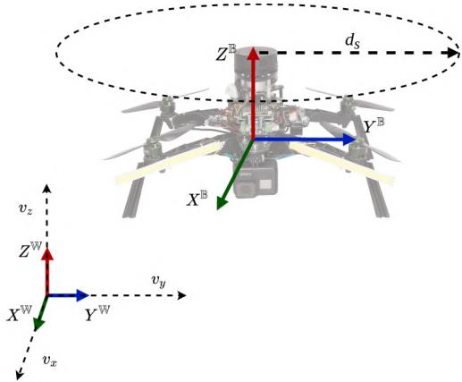
Fig. 1. Utilized coordinate frames, where  $\mathbb{W}$  and  $\mathbb{B}$  denote the world and body coordinate frames, respectively. In addition, the safety distance around the UAV is denoted  $d_s$ .
