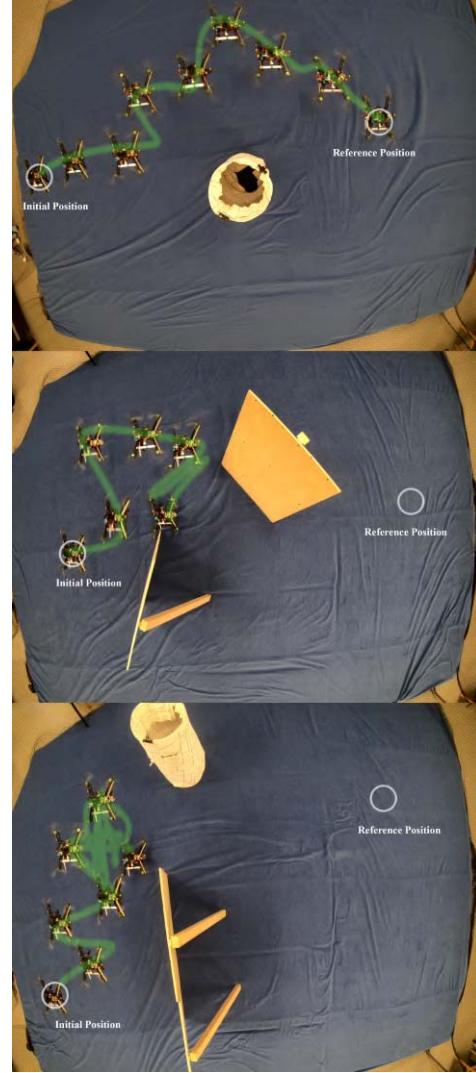
Fig. 26. Paths produced by the baseline APF for the three experiment scenarios. The scheme is incapable of completing the last two obstacle courses due to overly aggressive maneuvering.
