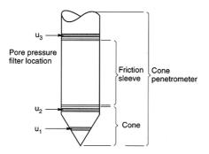
Fig. 3. The schema of cone penetrometer [10]
