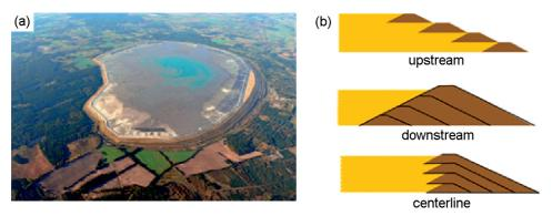
Fig. 1. a) Overview of Zelazny Most TSF. b) TSF construction methods: upstream, downstream, centerline
