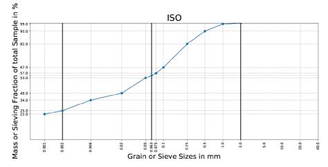
Fig. 5. The example of grain size distribution curve
