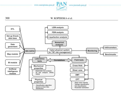
Fig. 2. Main functional modules of a cyber-physical system dedicated to the security of TSF
