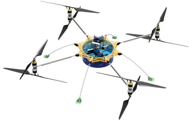
Fig. 4. Mars Coaxial Quadrotor (MCQ) used for the exploration mission.
