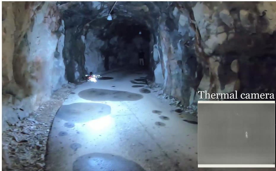
Fig. 4: UAV performing a full autonomous search and rescue mission, based on an onboard thermal camera video feed <https://youtu.be/0gvXjWbPLOA>.
