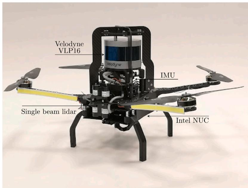
Fig. 9. The UAV used for the 3D path planning experiments.
