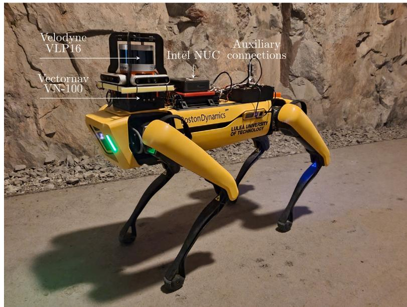
Fig. 8. Spot equipped with the attached sensors for the autonomy navigation and computational power. In this view perspective, the Vectornav IMU is placed under the Velodyne lidar and is not visible in the Figure.
