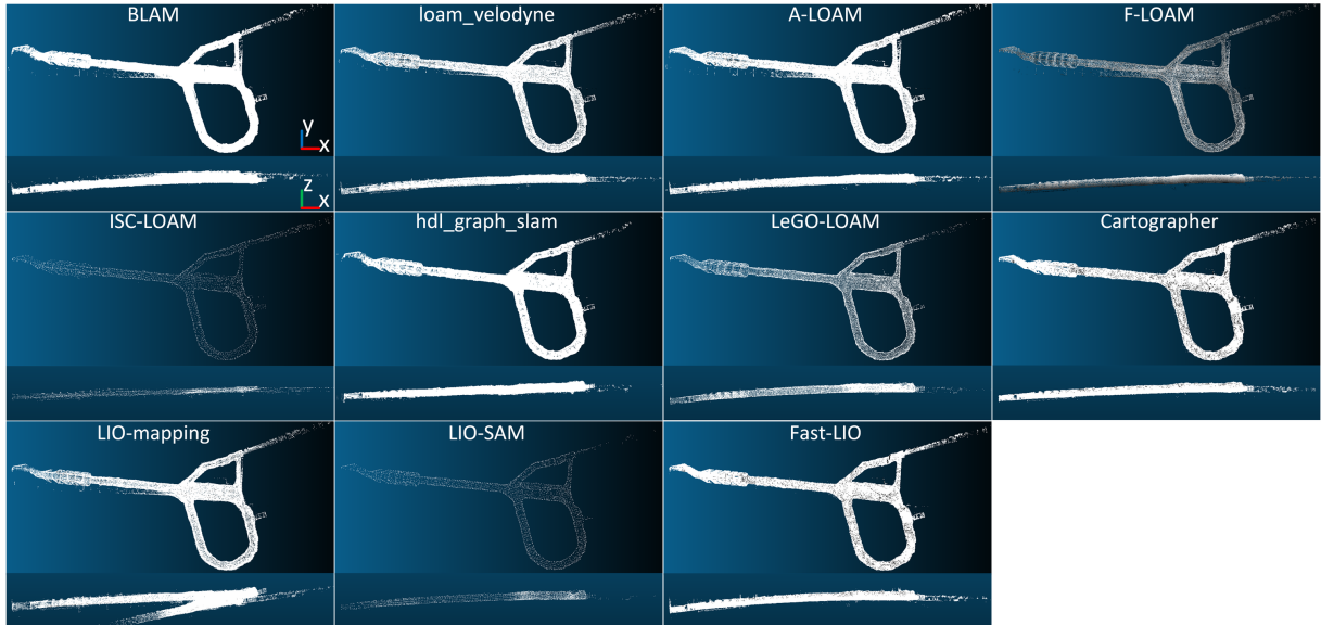
Fig. 5. Produced 3D point cloud maps from each method. The global coordinate frame for all figures is as defined for BLAM method, in which on the upper part is shown xy view and on the bottom xz view.
