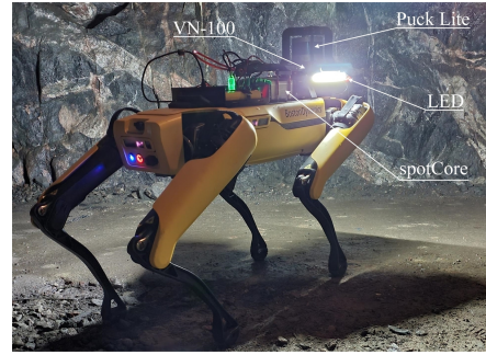
Fig. 1. Spot robot equipped with sensors for dataset collection in the underground tunnel.
